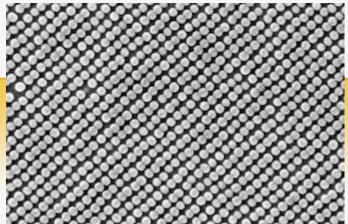
This pattern has 1.2 trillion dots per square inch, showing the dense patterns of magnetic islands made by HGST Labs using such emerging nanotechnologies as self-assembling molecules, line doubling and nanoimprinting. Each dot can store a single bit of data (Source: HGST).
