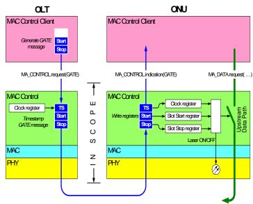
Figure 7: Path of GATE Message from OLT to ONU
