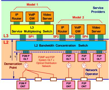
Figure 5: EPON in the Ethernet Access Model
