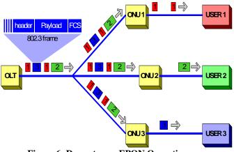
Figure 6: Downstream EPON Operation
