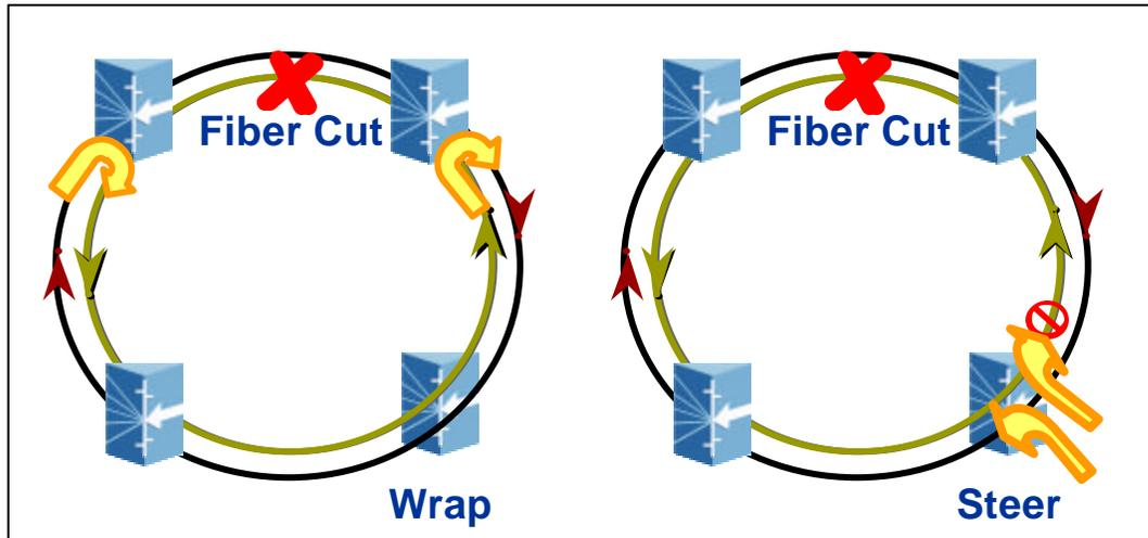
**Figure 2. Wrap and Steer Protection in RPR**
