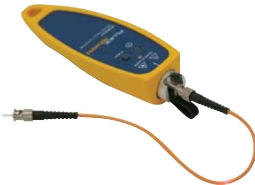
Figure 13: VFL used to locate a break in a patch cable. Note that light will not penetrate all fiber jackets at a break.
