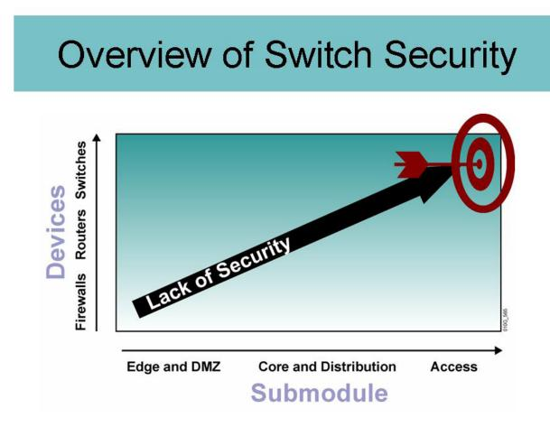
A firewall needs to be configured specifically to allow IP packets to traverse it. By default, routers do not filter traffic; however, they can be configured to filter traffic based on inspecting values in layer 3 and layer 4 IP headers. Switches can also be configured to thwart attacks launched at the LAN layer.
