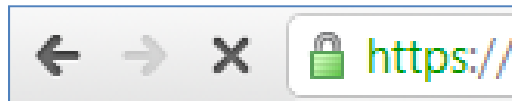
Figure 2.6: Visual cues, such as the lock and green-colored text can help to indicate to customers that a site has been authenticated and communication between the browser and the Web site are encrypted.
